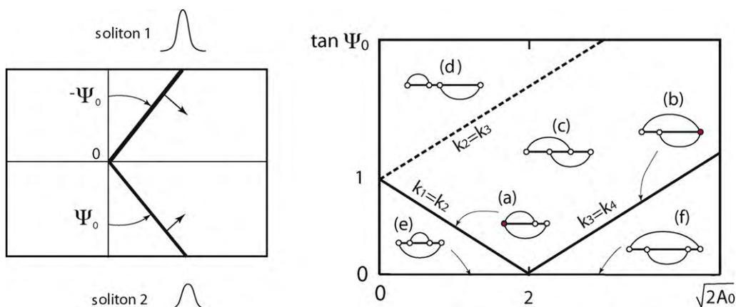
Fig. 14. V-shape initial waves. Each line of the V-shape is a semi-infinite line-soliton. We set those line-solitons to meet at the origin, and fix the amplitude of the soliton in  $y < 0$  to be 2.  $A_0$  is the amplitude of the soliton in  $y > 0$ . The right panel shows the incomplete chord diagrams corresponding to the choice of the values  $A_0$  and  $\Psi_0$ . There is no corresponding exact soliton solution on the dotted line of  $k_2 = k_3$ .
